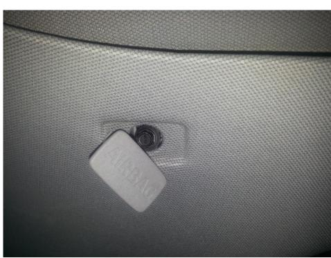
Use a flat bladed tool to release the retainer from the C-pillar panel.
