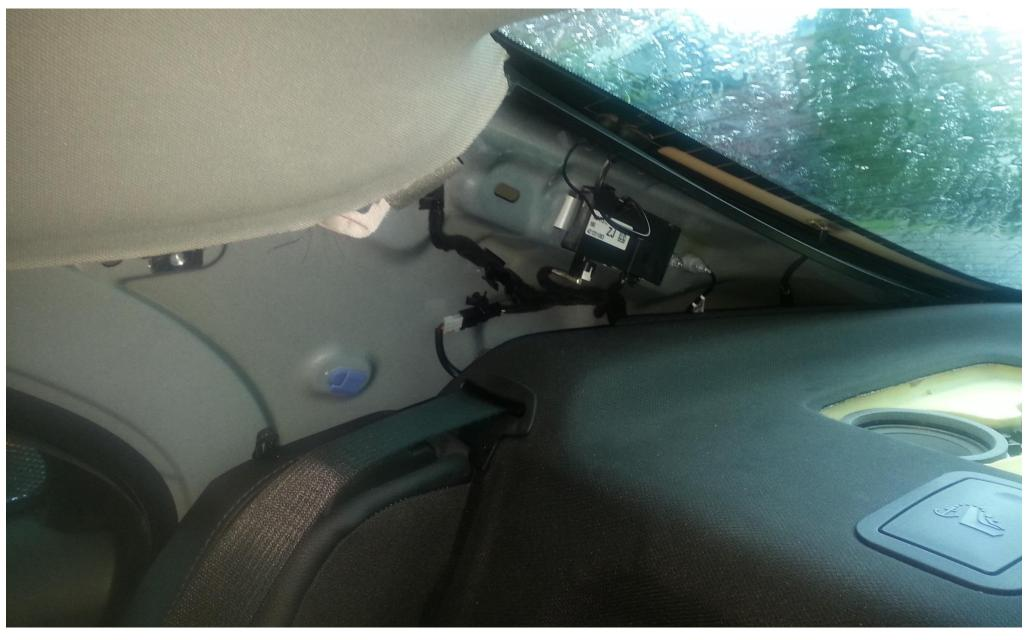
Disconnect the white electrical connector in the middle of the picture above (use a small flat bladed tool to unlock the connector).
